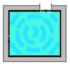
The roasting phase in which the goods get crispy begins. Now the flaps are opened to let the vapor escape. Dry, preheated air is blown via intake channel into the chamber. The flaps remain open until the basket has been emptied.
