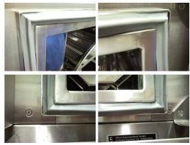
4. Push the seal into the notch. Start in the middle of each side and work your way to the corners. Make sure neither to stretch nor to forge the seal.
