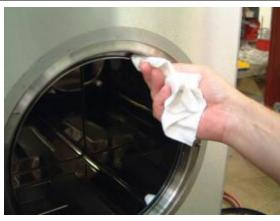
8. Put in the new seal. Place the splice of the seal in the middle of the upper notch.
