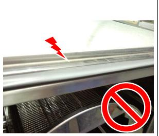
Insert lamella sheet and basketholder again. Close the door. Remove the old basket gasket by pulling it out.
