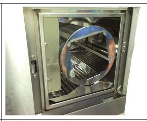
3. Assemble in the new seal. Start with the 4 corners.
