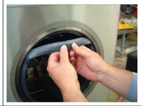
7. Clean the notch of the seal; remove grease and other residues.
