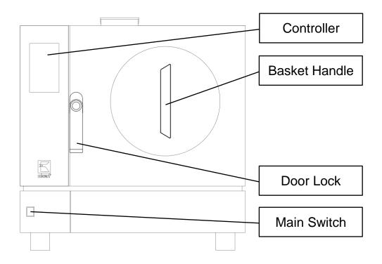
Computer control (Controller): The controller is used to control the complete cooking process
